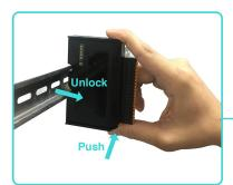
Unmount single modules easily with a push and unlock design
